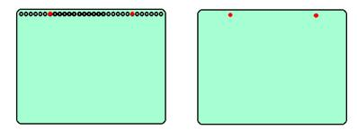
2. Check your pages are in order. Add pages to the split key rings. You may choose to close the opening on the ring after the pages are in place with a small piece of cloth duct tape. This stops the pages catching in the rings when in use.
